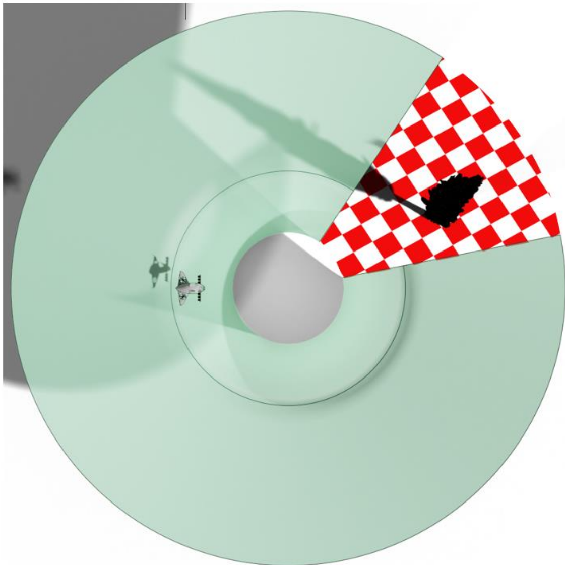
Figure D-20. Vertiport obstacle-free volume with omnidirectional approach and take-off climb surface and prohibited sector — top view
