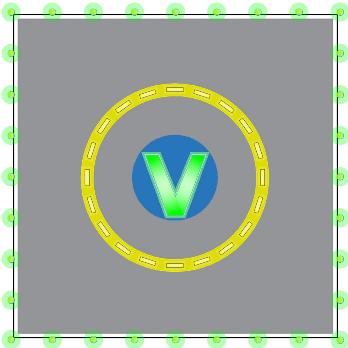
Figure E-35. Perimeter of a vertiport that is elevated, vertiport identification and TDPC lighting
